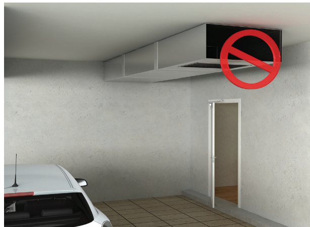
There should be no supply or return air registers in the garage
